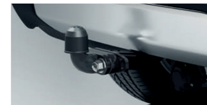
Towing System – Fixed Height Flanged Tow Bar Fixed position tow bar, tows a trailer up to 2,500kg load capacity for 5 seat.
