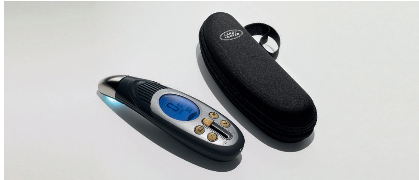
Tyre Pressure Gauge Digital tyre pressure gauge which stores recommended pressure and has a 360° rotating nozzle to locate tyre valve, LED light to locate tyre valve, tread depth gauge to measure tyre tread depth, measuring in psi, bar, kpa, kg/cm 2 . Range 0-99 psi/0-7 bar and comes complete with storage case.
